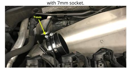
**Step 15**Insert intake tube into in the carbon fiber airbox top.
