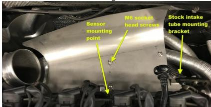
**NOTE**: For the 4" tube version, depending on what turbo inlet is being used (stock or 4" aftermarket), the 034Motorsport heat shield may need a little tweaking/bending to clear the assembly at the tube.
